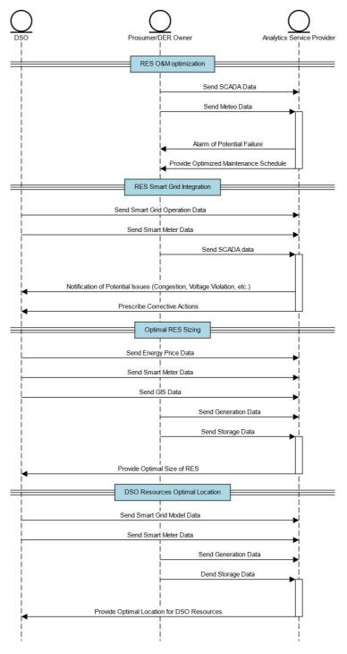
Figure 7 - Sequence diagram for the use case #5.
