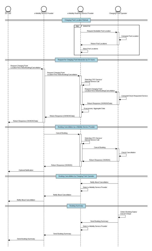
Figure 6 - Sequence diagram for the use case #4.
