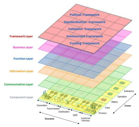
Figure 14 - SGAM plus: the 6th layer "Framework" (from [7]).
