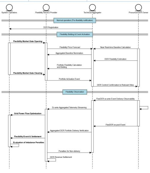
Figure 4 - Sequence diagram for the use case #2.
